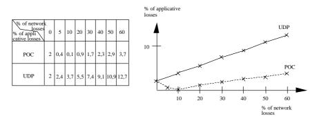
Figure 8. Comparative assessment of losses with POC and UDP for PNSVS
