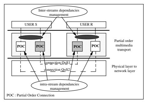
receiving transport entity (Figure 5) integrates a manager for multimedia multiconnections [CHASSOT 95C].
