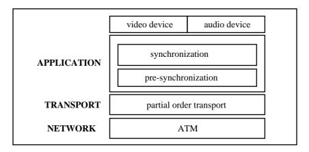
Figure 9. PNSVS architecture on top of a partial order transport service
