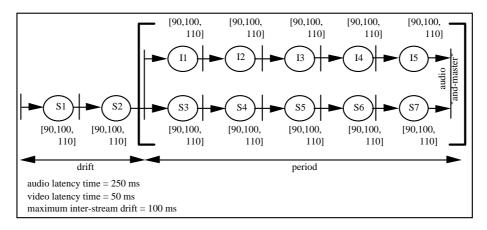
Figure 2. Applicative TSPN taking into account the hardware latency times
